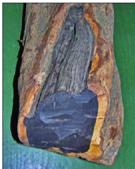
Dried, cut log, about 8" in diameter. The dense, blackish-purple heartwood is in sharp contrast with the straw-yellow sapwood. Logs are often riddled with defects, such as ingrown buttresses, heart rot, hollow pockets and checks, which make it difficult to obtain completely sound wood for woodworking purposes such as carving and the musical instrument trade.
